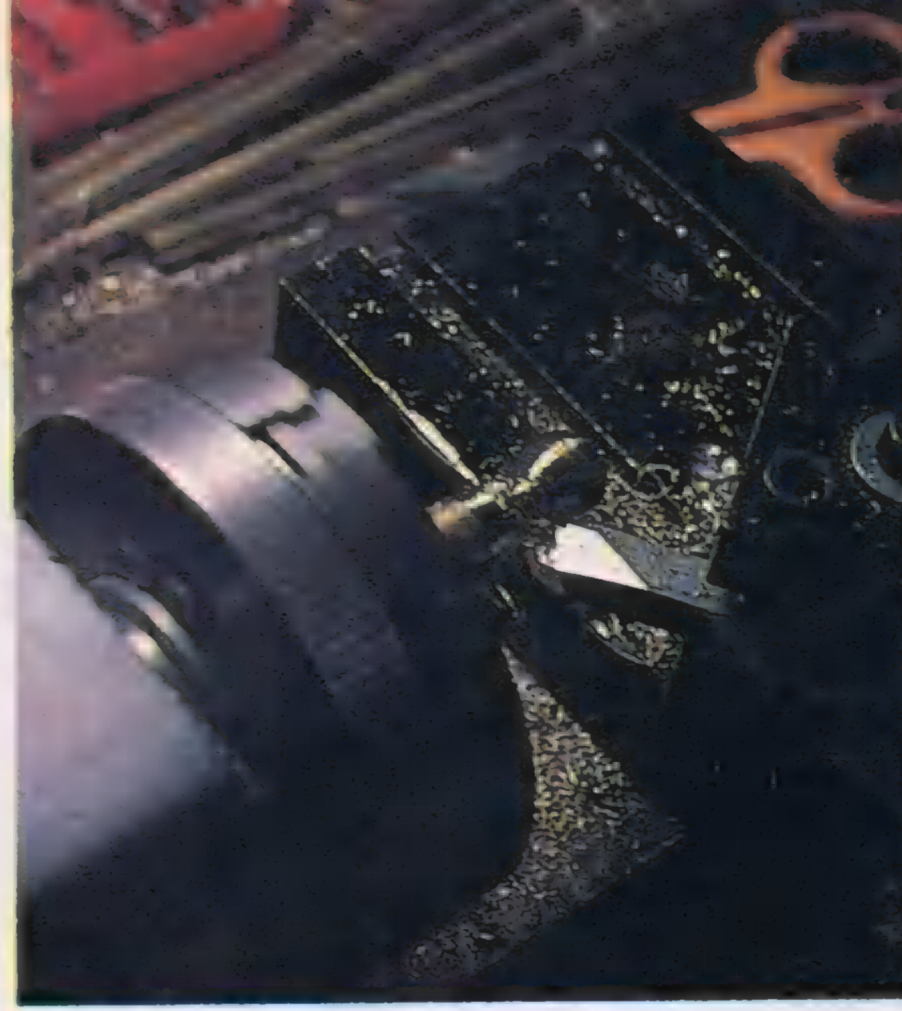
The third cut in the rod is made with a cutting bit.
